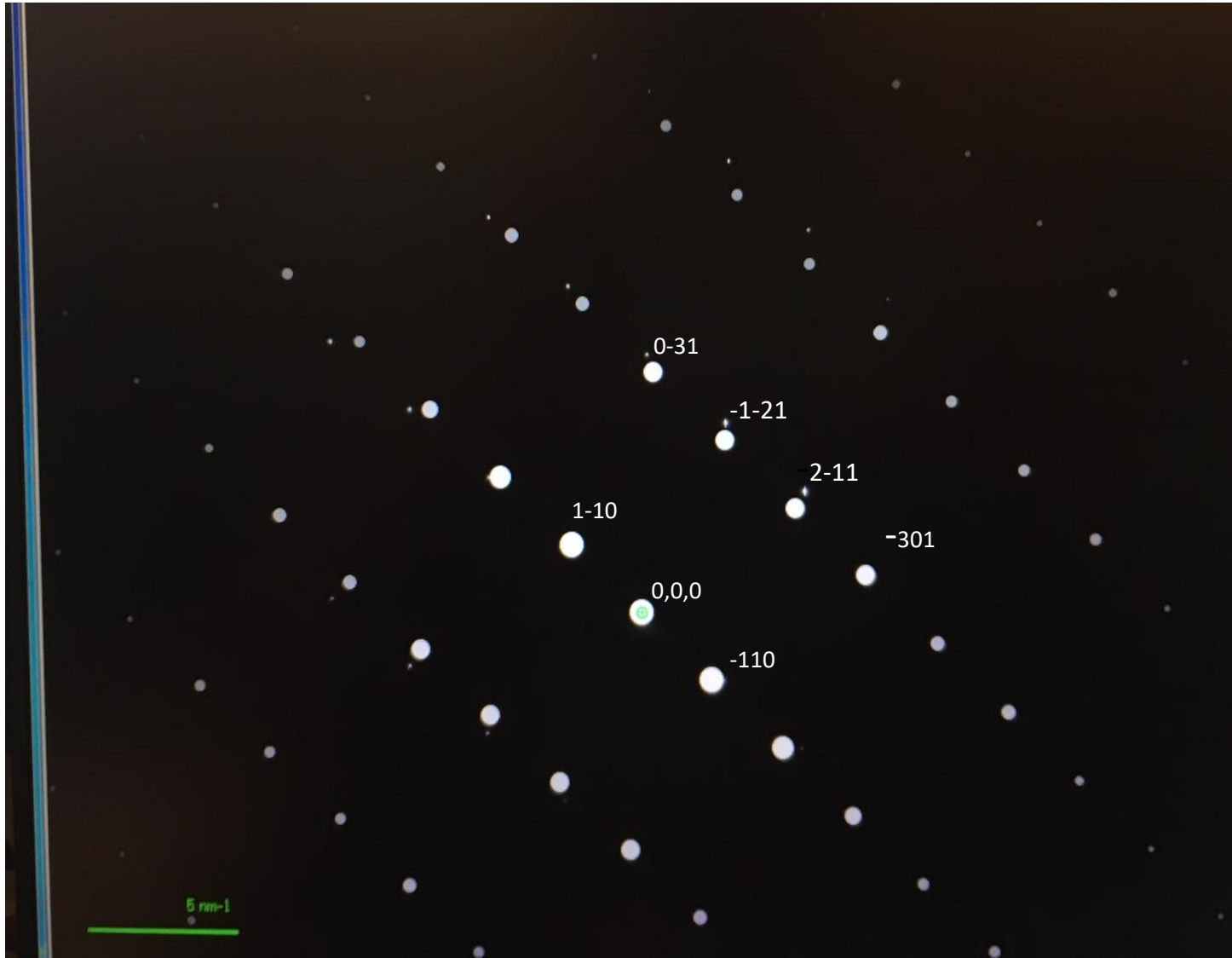
Figure A 3.7 JEMS simulation of Rutile in \langle 113 \rangle zone axis. With the pattern indexed consistent with Weis' zone law and the distances measured
