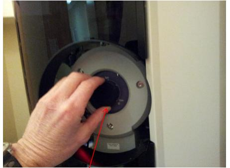
When time reaches 0, insert rod by turning Counter Clockwise and letting it gently into the Titan.
