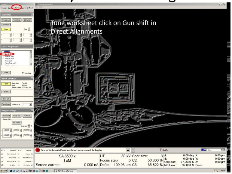
Beam and Gun Shift align\*, we flip between spot 6 and spot 2
