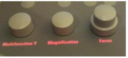
Computer auto assigns gun shift to Multifunction x and Multifunction y. Use MFx and Mfy to center beam at spot 2!
